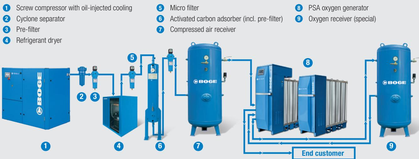
All from a single source: As a system provider, BOGE supplies you with an optimally tailored complete system comprising a compressor, filter, refrigerant dryer, activated carbon adsorber, compressed air receiver, oxygen generator and oxygen receiver. The result: Security of supply, independence and economic efficiency.
