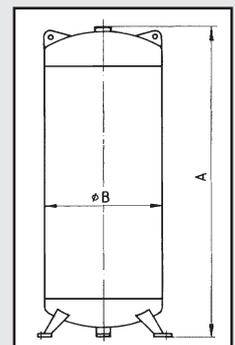
Oxygen receiver manufactured according to directive 97/23/EC, with CE symbol, incl. safety valve and accessories.
